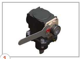
Insert spindle wrench behind collet nut. Align spindle wrench with the wrench flats on the spindle.
