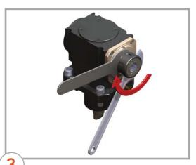
While holding the spindle wrench firmly, turn the collet nut wrench clockwise to tighten.
